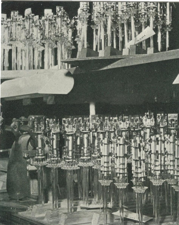
GUN ASSEMBLIES stand in soldierly array, having been painstakingly inspected for imperfections before being passed on to the next production technician. Final adjustments are made here before sealing the gun to the bulb.
