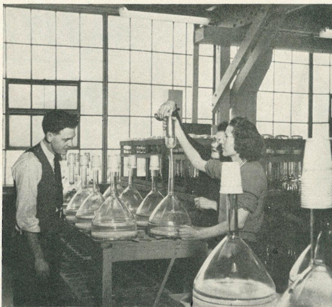
ALBERTA ZELASKO and Mrs. Margaret Summerson pour an aqueous suspension of phosphor into the tubes while Fred Larson looks on. The phosphor settles out to form the screen. The liquid is then siphoned out and the cathode ray bulb baked before assembling.
