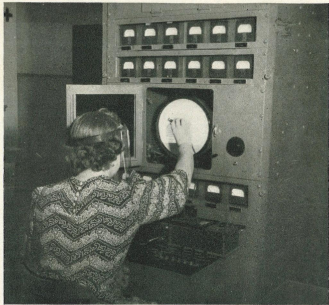
EXACTING TESTS are an essential part of production. Here, Mattie Carlson checks screen brightness with a portable photo cell. This is only one of a large number of tests made on each cathode ray tube in order to insure the highest standard of quality for our customers.
